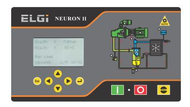
Elgi's Neuron II is a high end RISC microcontroller for control of medium to large screw air compressors. The system allows you to monitor and control overall system performance with service indications, malfunction alarms and safety shutdowns. It also includes a service and operational history feature to provide real-time feedback and increases system productivity
